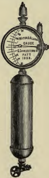
FIG. 26. LANE'S LOW WATER AND ALARM GAUGE.
